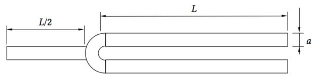
You will create a tuning fork model in two and three dimensions which adhere to the specifications given below, and then carry out several simulations. In each of these, you will determine the initial vibrational frequency of the model and the first nine overtones plus stresses. (Create a linear perturbation/frequency analysis step with ten modes using the "Lanczos" eigensolver.) I recommend using a = 4 mm and starting with L from 80–90 mm.
